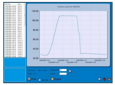
and observe how the value F0 (referred to  $121.11^{\circ}$ C) changes progressively. The process is carried out with Z=10:
