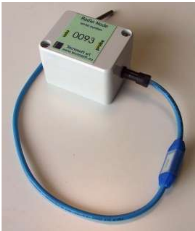
Temperature Intelligent Sensor with Radio Node: electronics of the sensor is incorporated in the cable.
