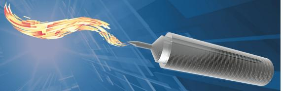
Temperature data logger from -40°C to 400°C (standard calibration from 25°C to 140°C, calibrable from -40°C to 400°C, only the probe will resist above 140°C) with 30 cm bendable probe, 2 mm diameter (first and last 30 mm cannot be bent). **Battery is user replaceable** and the data logger is **provided with a National Reference traceable certificate** on 6 points.
