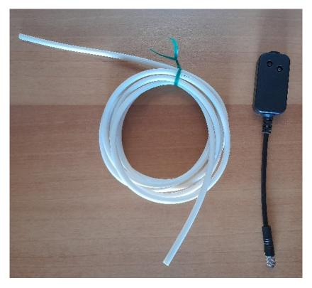
• On the differential pressure Smart Sensor case there are two pipe connectors: one generates positive signals (P+) and the other generates negative signals (P-). The output presents a signal which is the algebraic sum of the two pressures (positive if P + prevails and negative if P- prevails, zero if P + and P- have the same absolute value, and negative if P- prevails).
