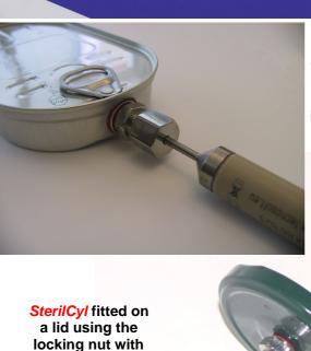
the possibility of adjusting its depth inside the jar, in order to reach the product's core SterilCyl fitted on a tin of canned fish; shows use of the locking nut and the threaded insert on a sharply curved surface
