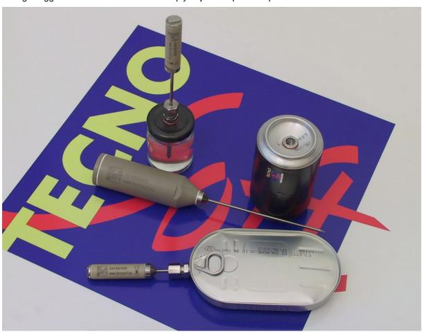
The range of applications catered for by the new Fastening System for Tecnosoft temperature data loggers; for reliable and improved monitoring of food processes employing different types of containers and materials, including pressurized cans.
